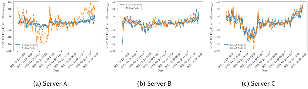
Fig. 21. DRAM decay traces from three f1.16xlarge instances (24 FPGAs in total) for a period of 24 hours, using the differences between successive measurements c_{diff}^i as the comparison metric, which results in the highest co-location accuracy of 96%. Within each server, measurements from slots in the same NUMA node have been drawn in the same style.
